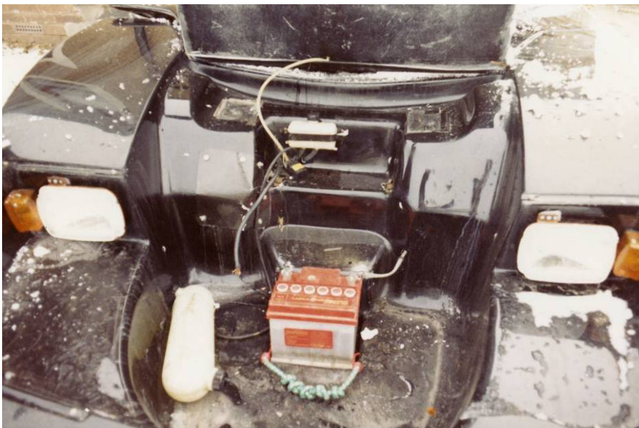
View of the front compartment after the accident: This picture shows some of the detail described earlier. Here you can see the steering box cover plate, the windscreen washer installation, Brake fluid master cylinder and the battery.
