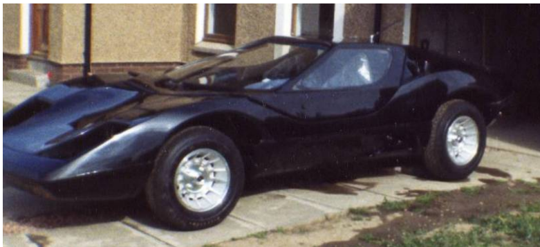
View of the car after lowering the rear suspension
