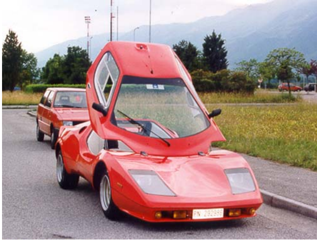
Puma GTV – Note the canopy Hinges from the front on this car
