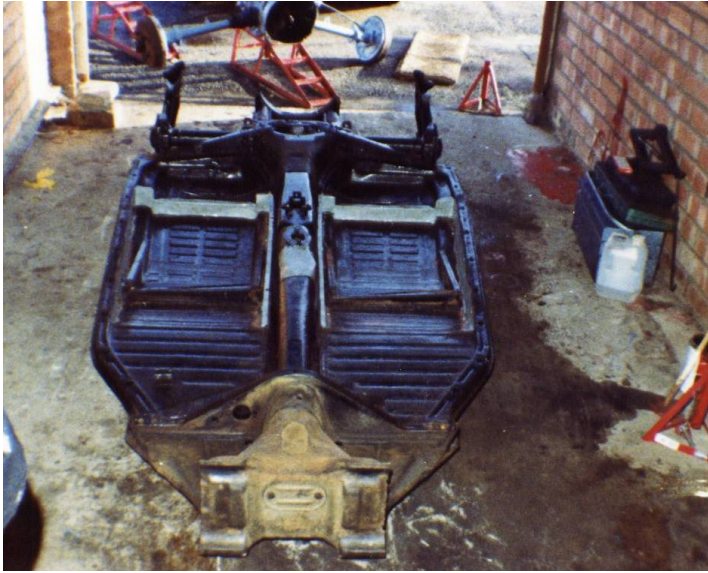
View of the floor pan with lowering panels in place (light grey in colour).
