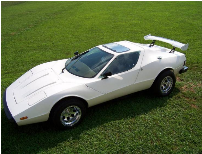
Sebring – Note the higher roof line – smoothed out sides and different front bonnet. The roof canopy also cuts deeper into the main body tub (Photo courtesy of owner Paul Hawkins)
