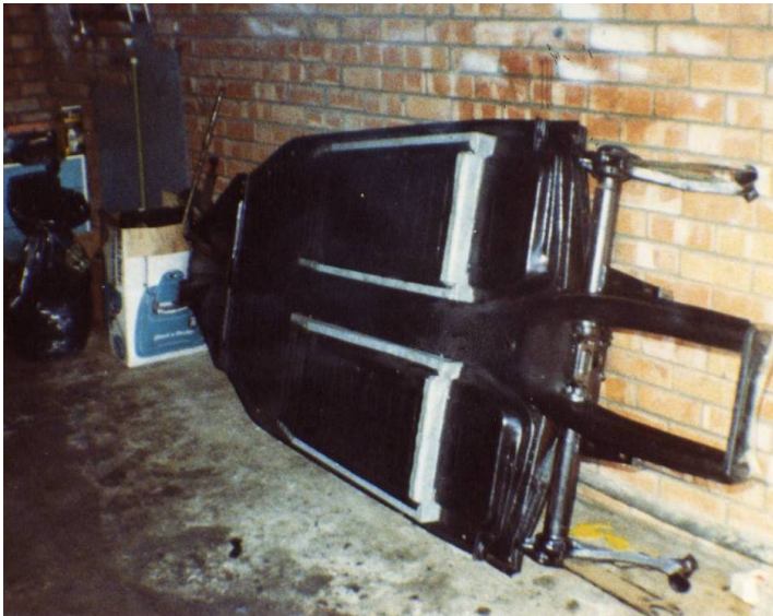
View of underside with lowering panels in place.
