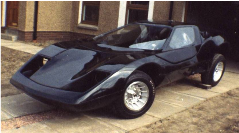
Views of the car with wheels fitted. Note the rear wheels still need to be de-cambered as the car sits high due to the lighter bodywork.
