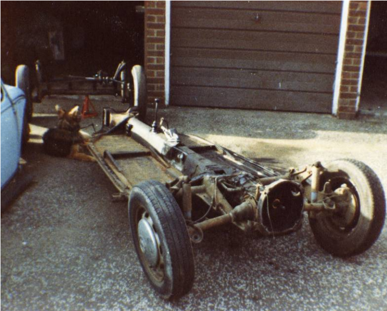
Complete rolling chassis after removal of body shell
