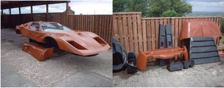
This series of photographs show the fiberglass components making up the basic kit
