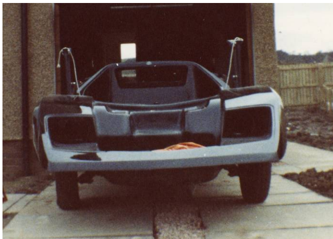
View of Body shell now permanently in position on the floor pan
