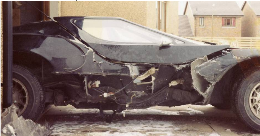
Side view showing the damage to the Nova
