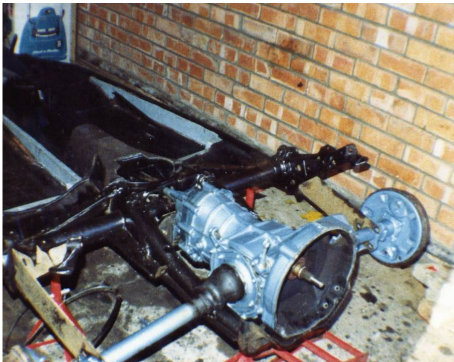
Transaxle assembly in position in the floor pan (this picture must have been taken at a period earlier than just described as you can see that the lowering panels have not yet been painted).
