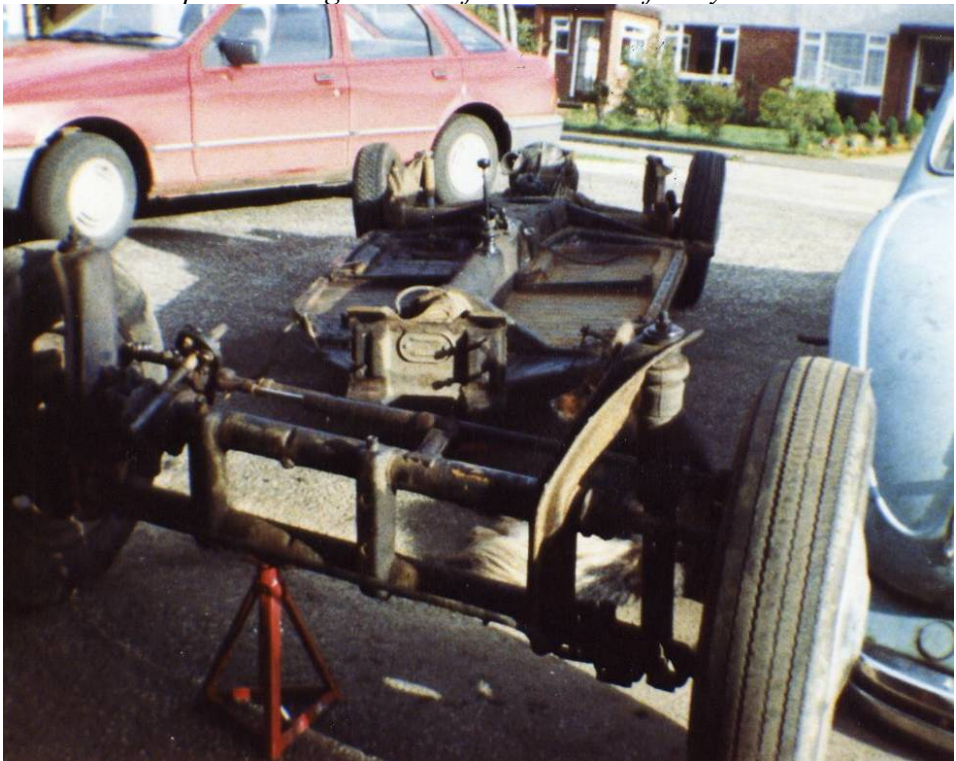
Another view of the rolling chassis – In both pictures you can see that the front axle assembly has already been unbolted from the rest of the assembly as described next
