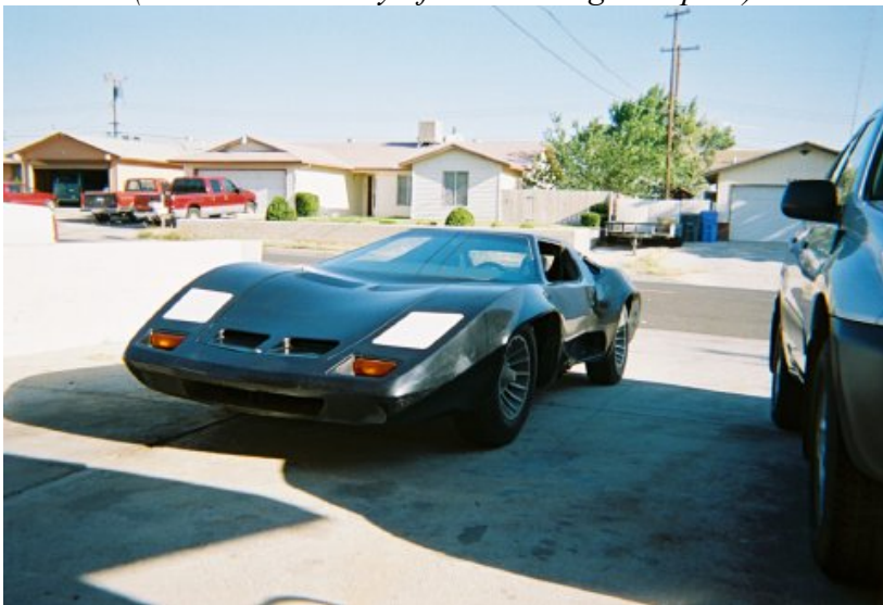
Sovran – Note the squared off wheel arches and changes to the front of the car
