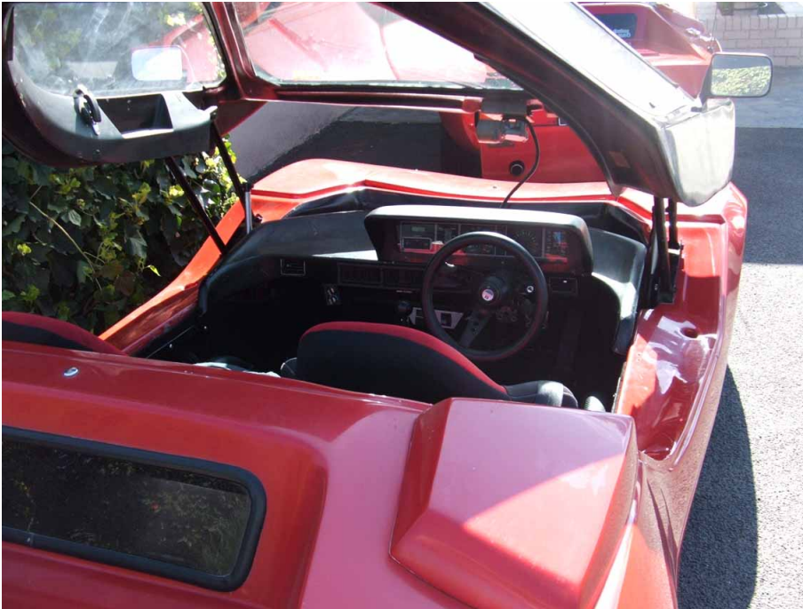
Eureka Canopy showing the groove around the body which is unique to the Eureka
