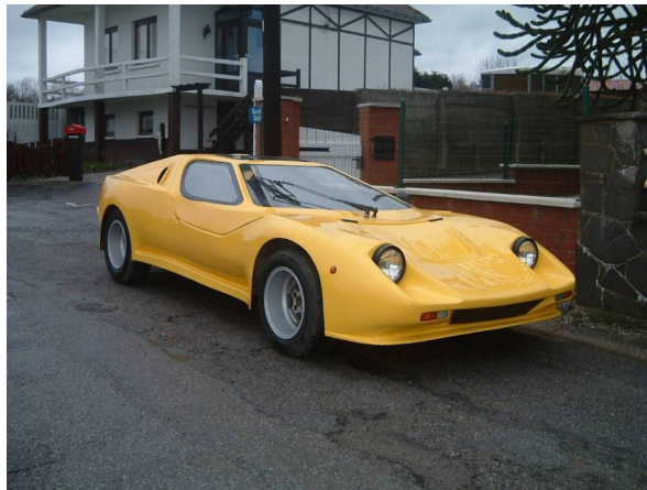
A later version of The “Puma” – Radically different from the Nova with upright round headlamps and similar “silhouette” though completely re-designed main body tub. The Roof panel is the only feature that is instantly recognisable as Nova
