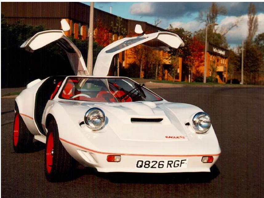
The Eagle SS – This is a Cortina based version as can be seen by the central hump on the front bonnet. The rear engined Beetle based kit looked very similar but without the pronounced bonnet bulge required by the Ford based car.
